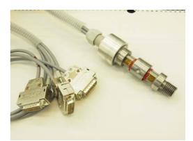
Fig. 3. Measuring bolt with installed strain gauge
